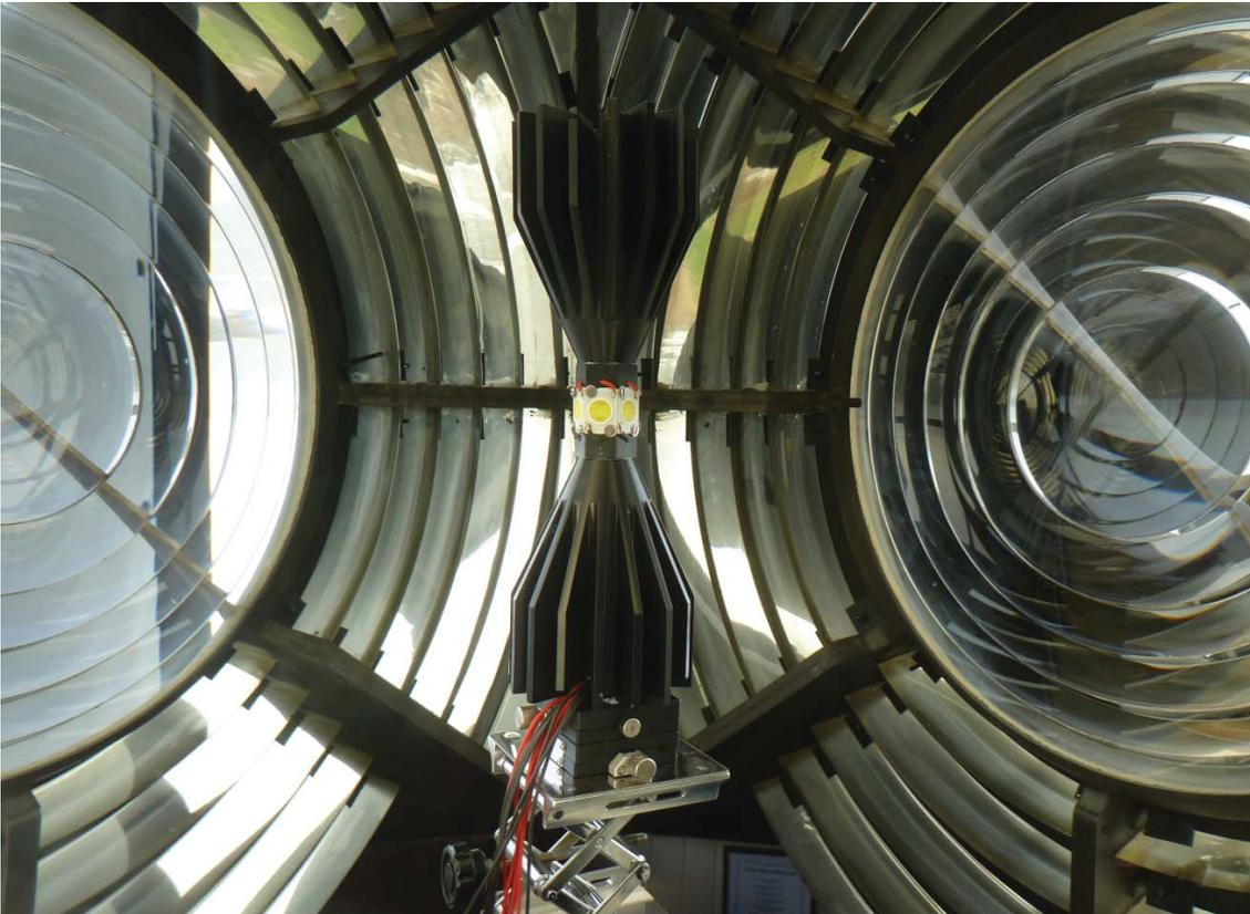
*Research and Radio Navigation - LED LIGHT SOURCE BEING TESTED IN A LIGHTHOUSE OPTIC*
